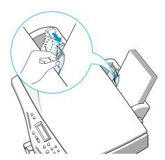
**5** If the paper jams as it exits to the paper output tray, remove the jammed paper by pulling gently on the paper.
